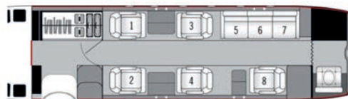
Cabin layout of a Hawker 800 series midsize private jet in an 8-seat configuration with divan.
